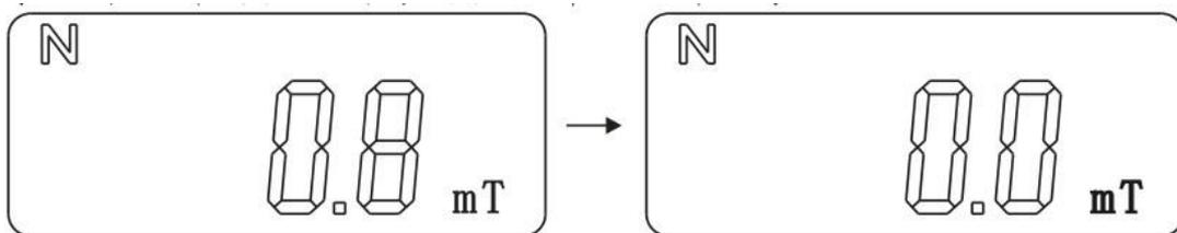
**Note:** Afterwards, change the measurement range or transform the AC/DC mode, you all need to reset zero.
