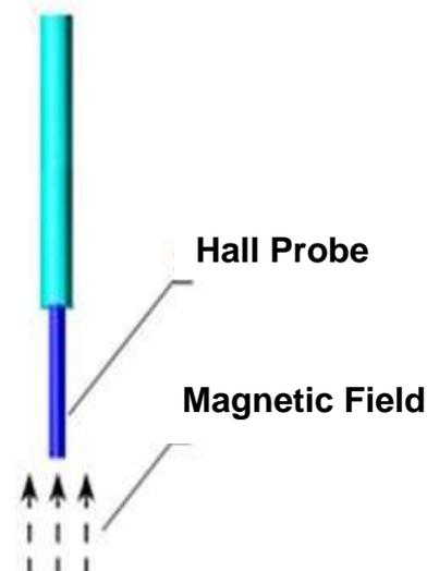
**Fig. 2: Axial Probe**
