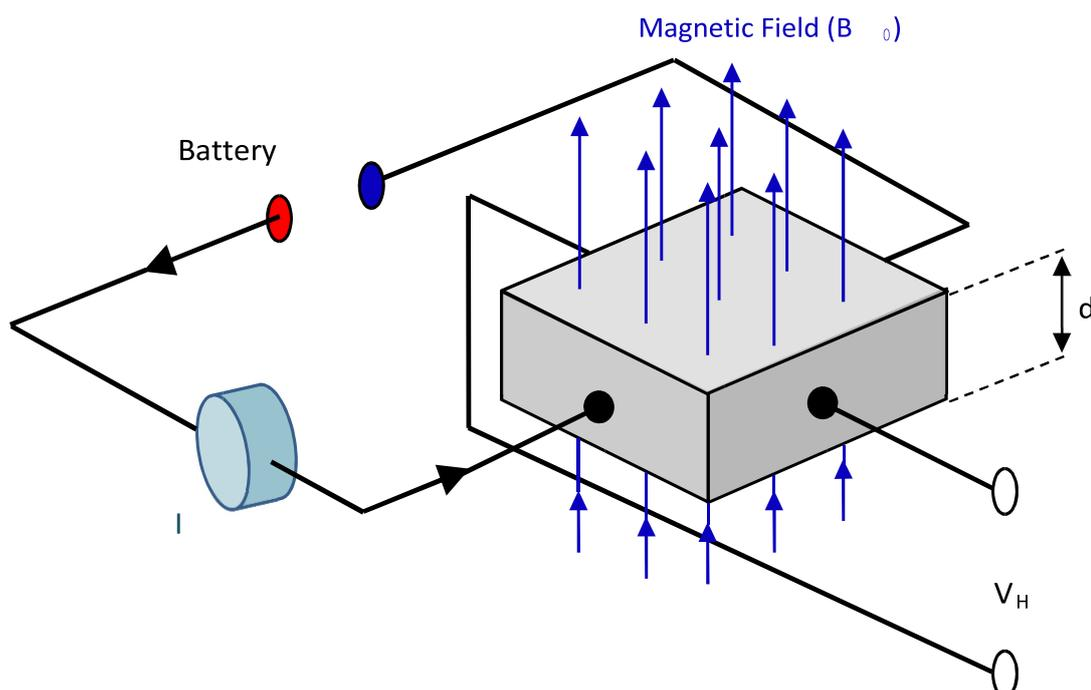
When placing the semiconductor carrying current in the magnetic field axial to the current direction, the semiconductor will generate a transverse Galvanomagnetic phenomenon, namely an electromotive force in the direction axial to the magnetic field and current, which is the Hall Effect.
