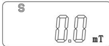
4. Select a suitable measurement range. Press the key RANGE switchover again and again, the measurement range should be transformed within 0~200 mT or 0~2000 mT.
