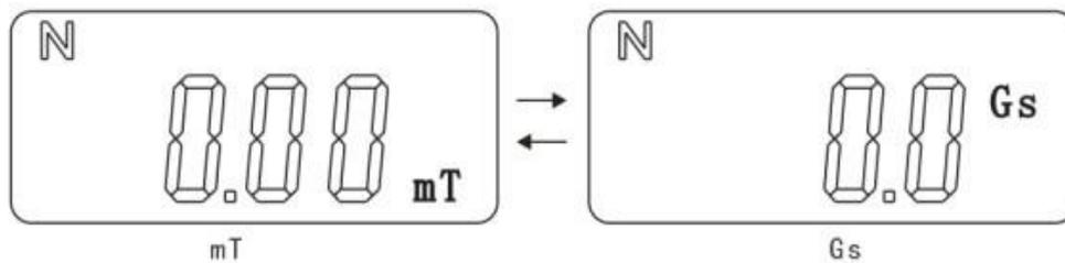
7. Resetting zero. Keep the sensor as far away as possible from the magnetic field. If the display screen does not show "000".you must press the key (3) to adjust it to zero.
