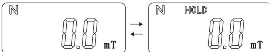
9. Loosen the cap of the Hall probe (see upper Fig). Place the Hall probe touching the surface of the material tightly (DC magnetic field) or at the zone of the measured magnetic field. The screen (1) will show the value of the magnetic field.
