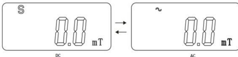
6. Selecting the unit of display. Press the key (7) of conversion, the display unit should be transformed from mT to Gs.
